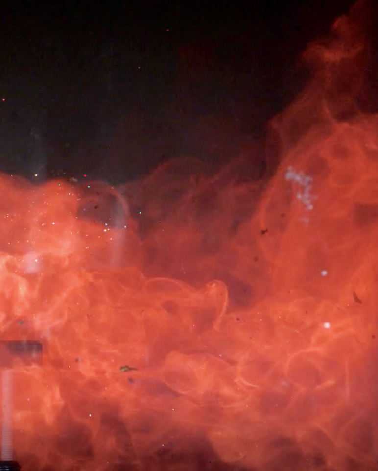
Section from a video recording of the bullet impact of an exemplarily selected lithium-ion bicycle battery (dimensions: 38 centimeters by 8.5 centimeters by 8.5 centimeters).
