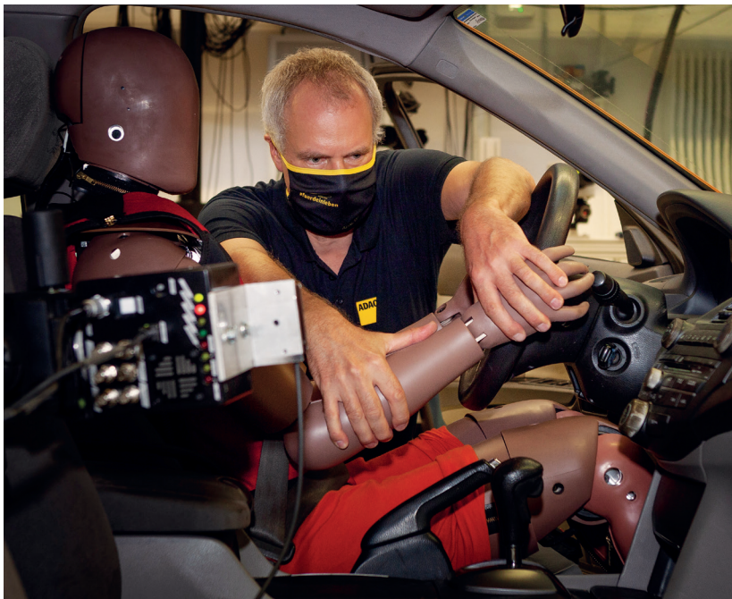
The dummy THOR-50M is being adjusted for the crash test under X-ray.
